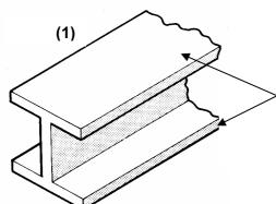
The advantage of **I** beams is that most of the material is placed where the highest stresses (1) are - at the outer edges. (1)
